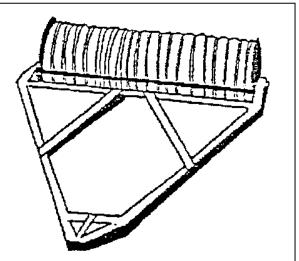
Another homemade roller: close the ends of a culvert and install a tow-bar.
