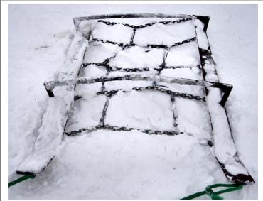
K'atl'odeeche First Nation ski trails are levelled and renovated with a home-made chain drag. Chains are welded to old 'Cat' blade runners and tightened with turnbuckles.
