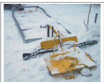
One Pass Grooming: the Norman Wells Ski Club groomer drags a 'bed-frame' leveller and track-setter in tandem. The snowmobile does the packing.
