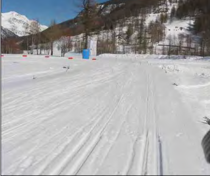
Track is removed prior to intersections, such that sit-skiers can move over to inside corner.
